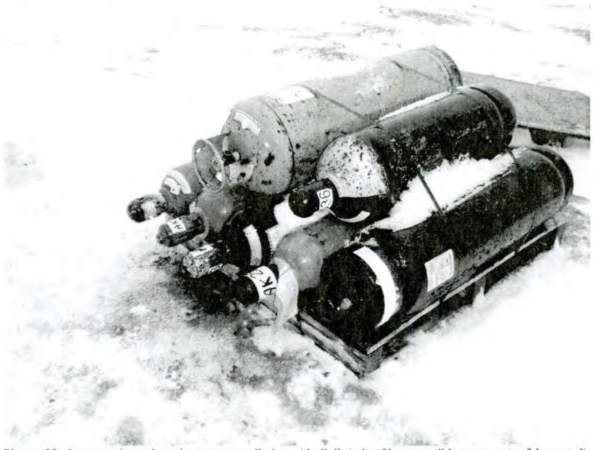
Picture 25 : Improperly packaged empty gas cylinders, Akulivik (mix of incompatible gases, not safely crated)
