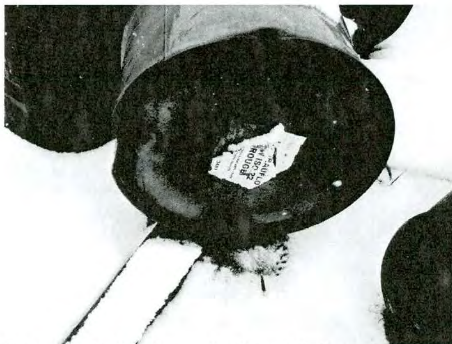
Picture 22 : Leaking barrel in garage barrel storage, Kuujjuaraapik
